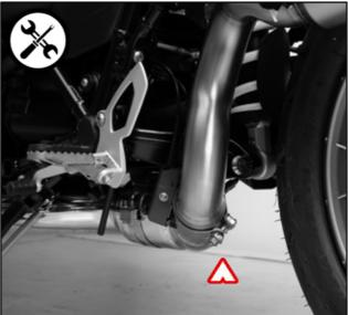
Remove the stock muffler.
