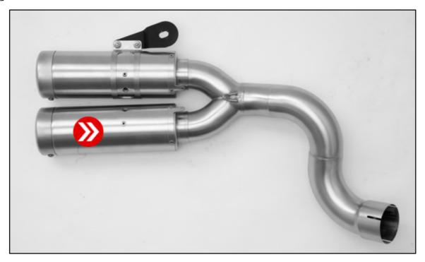
Mount the supplied exhaust bracket with the supplied hex socket screws to connect the two mufflers. Hook the two springs.
